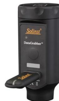
One push-button is used to download all of the data in a Levellogger's memory to a USB device plugged into the DataGrabber. A convenient LED light indicates the operation of the DataGrabber. The data in the Levellogger memory is not erased, and logging is not interrupted if the Levellogger is still running. The DataGrabber uses its own replaceable 9V battery.
